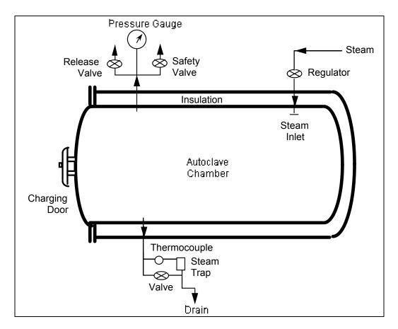
Figure 6. Typical Autoclave Treatment System
