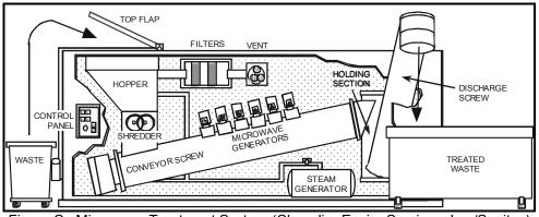
Figure C. Microwave Treatment System (Chevalier Enviro Services, Inc./Sanitec)
