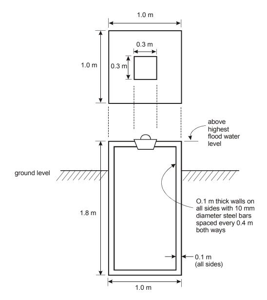
Figure 7. Basic Concrete Septic Vault Design
