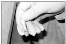
Photograph 25. Remaining Plastic Portion of the Syringe After Treatment in the Needle Destroyer
